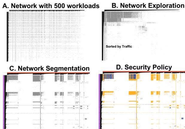
Figure 2: Develop Segmentation Strategies: Sub-Fig. A shows an unsegmented network, in Sub-Fig. B nodes have been sorted by the traffic volume for each node. In Sub-Fig. C, we demonstrate logical segments created by the security analysts. And in Sub-Fig. D we show that security analyst secures communication between workloads based on network segments.
