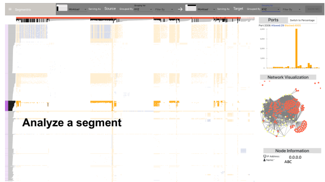
Figure 3: Segmentrix supports interaction to analyze segments. In this figure, the user has selected a segment to analyze. The selection highlights the source segment and all the connected target segments. For context, we also display the node-link visualization of the selected segments.
